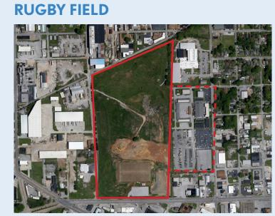
A local sports club offered financial support to further cap portions of the site. In exchange, a rugby field is constructed on clean fill on the southern portion of the park. Additional capping of 24" of clay topped with 12" of vegetated cover is installed on site in zones which the cap is deemed insufficient. The Sculpture Fields non-profit was formed in 2012.
